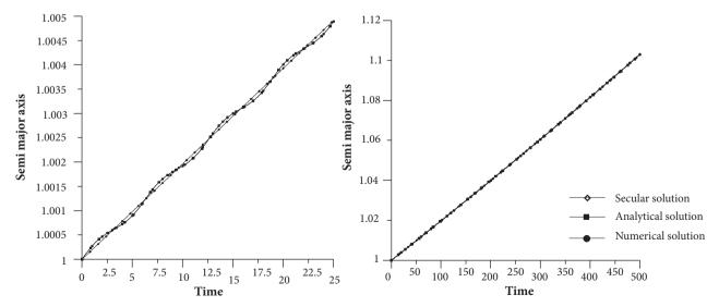
Figure 2. Comparison between secular, analytical and numerical time evolution of semi-major axis for maneuver 1 with  $t_r - t_n = 25.0$  and  $t_r - t_n = 500.0$ .
