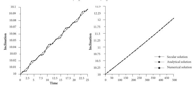
**Figure 4.** Comparison between secular, analytical and numerical time evolution of inclination of orbital plane for maneuver 1 with  $t_t - t_0 = 25.0$  and  $t_t - t_0 = 500.0$ .
