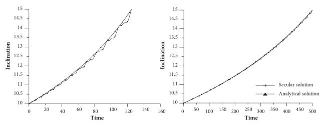
Figure 16. Secular solution and complete analytical solution of the TPBVP for maneuver 3 for both transfer durations – evolution of inclination of orbital plane.
