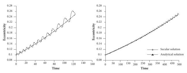
Figure 15. Secular solution and complete analytical solution of the TPBVP for maneuver 3 for both transfer durations – evolution of eccentricity.
