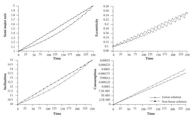
**Figure 11.** Time evolution of state variables for maneuver 3 with  $t_t - t_0 = 250.0$ .
