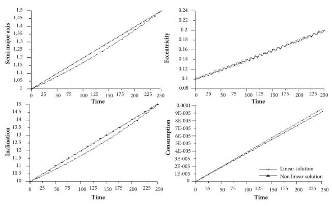
**Figure 13.** Time evolution of state variables for maneuver 7 with  $t_f - t_0 = 250.0$ .
