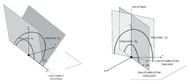
Figure 1. Geometric configuration of the initial orbit and the final orbit: (a) represents the maneuver with change in the inclination of the orbital plane and (b) represents the maneuver with change in the longitude of ascending node.
