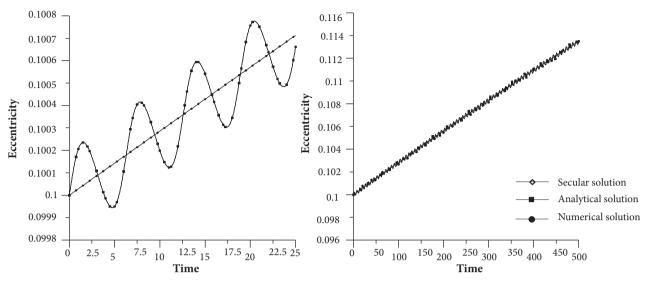
**Figure 3.** Comparison between secular, analytical and numerical time evolution of eccentricity for maneuver 1 with  $t_{t} - t_{n} = 25.0$  and  $t_{t} - t_{n} = 500.0$ .
