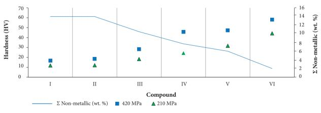
Figure 7. Vickers hardness after sintering.
