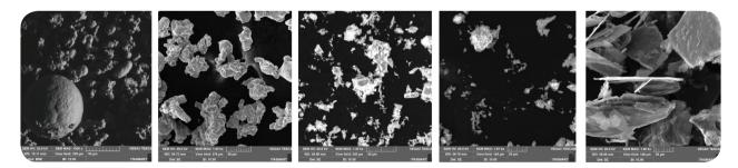
**Figure 3.** Particle analysis of (a) copper, (b) iron, (c)  $SiO_2$ , (d)  $ZrSiO_4$ , and (e) graphite.
