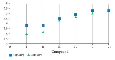
Figure 4. Sintered density.
