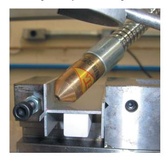
Figure 1. Experimental setup showing aluminum parts fixed at the bench. The white block is an alumina calibrated support, and the rounded nozzle is responsible for gas shielding.
