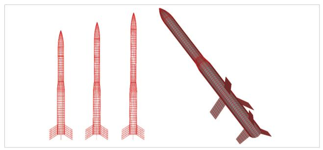
Figure 5. Aerodynamic meshes for the VSB-30 rocket for two stages configuration and four modules (right), and the single second stage for 2 to 4 modules (left).
