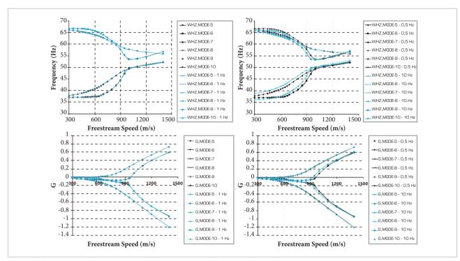
Figure 13. Evolution of the damping and frequencies as a function of the freestream speed.
