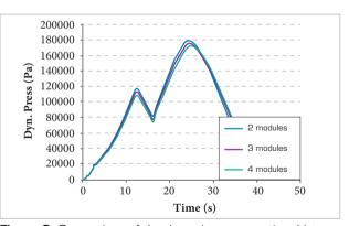
**Figure 8.** Comparison of the dynamic pressure time history for two, three and four payload modules.
