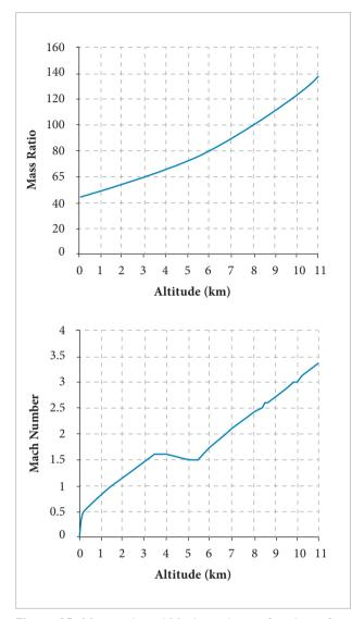
**Figure 10.** Mass ratio and Mach number as functions of the flight altitude.
