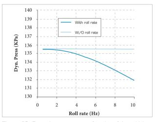
Figure 12. Dynamic pressure as a function of the vehicle roll rate.
