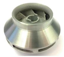
Figure 6. Printed and finalized experimental impeller, stretched and non-functional design, printed in one part.
