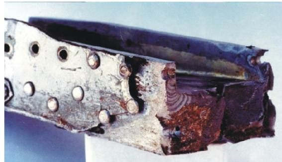
Figure 2: AT-26 wing main spar failure (Mello Jr., 1999).
