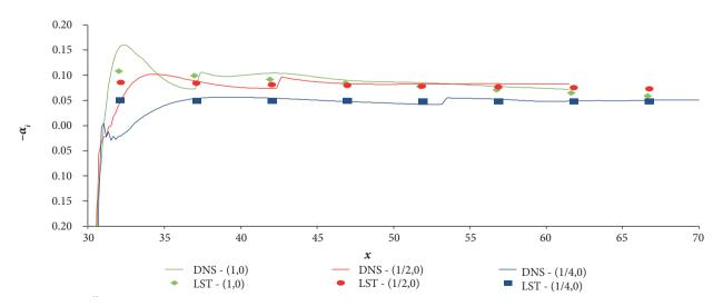
Figure 5. Spatial amplification rate in the streamwise direction. Comparison between LST and DNS for the 2D mixing layer.
