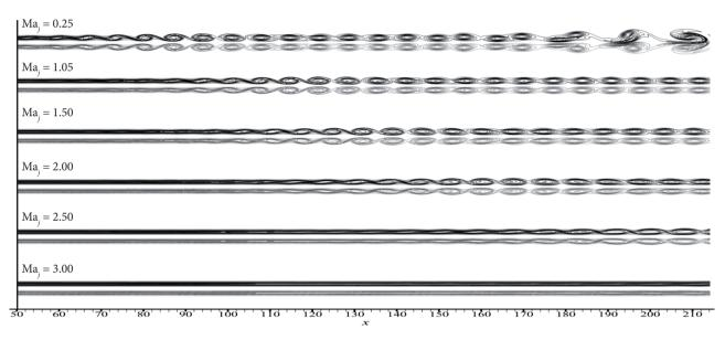
Figure 11. Spanwise vorticity for the 2D plane jet, varicose mode. Contour levels from -0.5 to 0.5. Solid lines for positive values and dashed lines for negative values.
