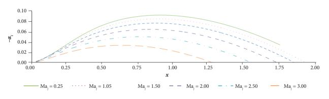
Figure 8. Spatial amplification rates for the 2D plane jet, sinuous mode.
