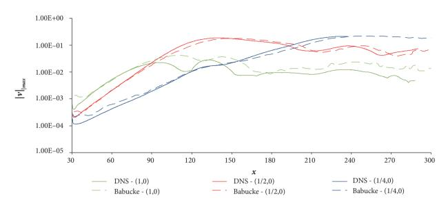
Figure 4. Maximum amplitude of v for each x position. Comparison with results from Babucke et al. (2008).
