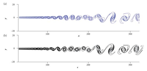
Figure 6. Spanwise vorticity contour levels from -0.26 up to 0.02 with an increment of 0.04. Results from (a) Babucke *et al.* (2008) and (b) DNS code.
