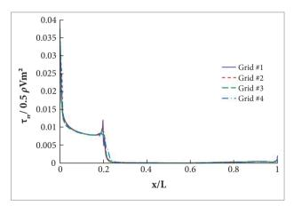
**Figure 3.** Comparison of the wall shear stress calculation for all tested grids.
