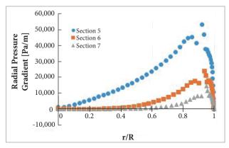
**Figure 11.** Radial pressure gradient for 3 geometry sections at S = 0.3 and  $2\phi = 24^{\circ}$ .
