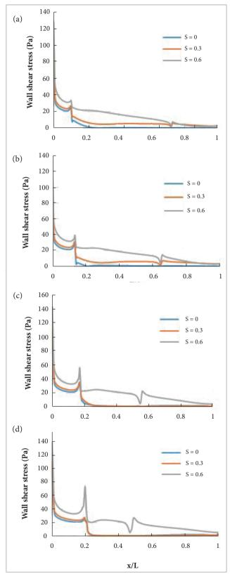
**Figure 14.** Wall shear stress along the diffuser length. (a)  $2\phi = 16^{\circ}$ ; (b)  $2\phi = 24^{\circ}$ ; (c)  $2\phi = 40^{\circ}$ ; (d)  $2\phi = 60^{\circ}$ .
