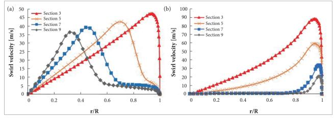
Figure 9. Swirl velocity profiles for  $60^{\circ}$ - diffuser. (a) S = 0.3; (b) S = 0.6.
