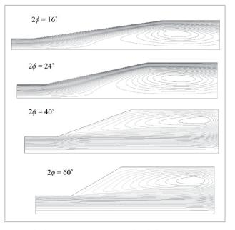
Figure 6. Streamline contours for S = 0.3.
