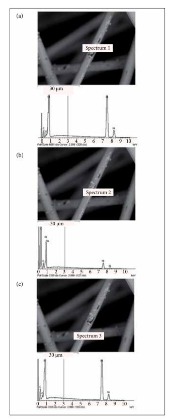
Figure 4. SEM/EDS analyses of the CF/Ni veil as received. (a) Spectrum 1, (b) Spectrum 2, and (c) Spectrum 3.
