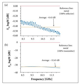
Figure 3. Curves of (a)  $S_{\rm 22}$  and (b)  $S_{\rm 24}$  versus frequency of the CF/Ni veil, as received.
