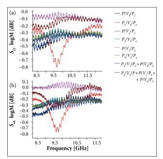
**Figure 7.**  $S_{22}$  (a) and  $S_{44}$  (b) parameters versus frequency for GF/epoxy resin/CF/Ni laminates.
