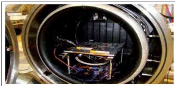
**Figure 8.** Coupons inside the LIT Thermal-Vacuum Chamber #1.
