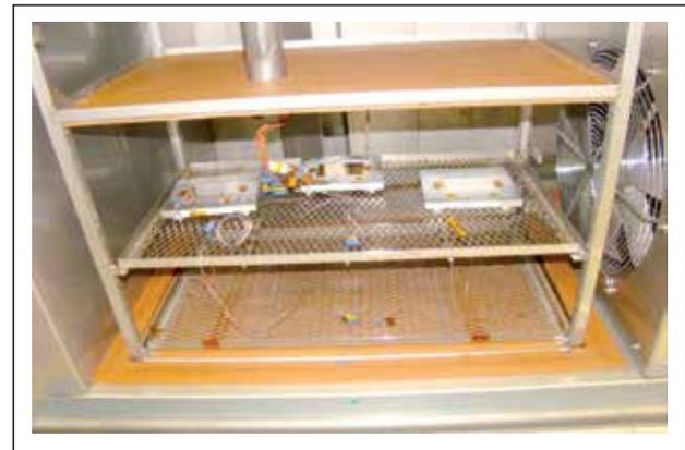
**Figure 11.** Coupons placed in the thermal-shock chamber elevator.
