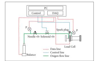
**Figure 2.** Diagram of the experimental apparatus. It is possible to see the data acquisition (DAQ); the control panel (PC), and the needle and solenoid valves (vlv).
