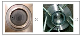
**Figure 4.** (a) Axial injector mounted on the test bench; (b) Large swirl attached to the test bench with the four oxidizer supply entrances.
