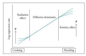
**Figure 7.** Diagram of the influence of radiation and kinetics effects on regression rates adapted from Altman (2001) and Pastrone (2012).
