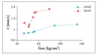
Figure 6. Regression rate versus oxidizer mass flux for each injection method.
