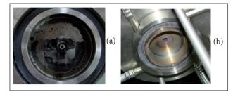
**Figure 9.** Comparison between injector cross-sections after firings. (a) Axial test; (b) Large swirl test.
