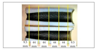
Figure 6. Cross-sections for the calculation of mean regression rate.
