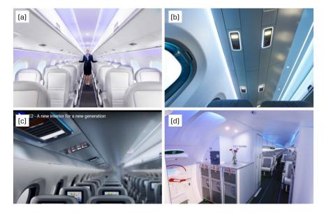
Figure 1. Different types of cabin interior lights. (a) Dome and wash lights of the Embraer E-jets E2 (Eden 2020).(b) Reading lights of the E-jets E2 Embraer (Airlines IATA 2014). (c) Warning sign lights of the E2 aircraft from Embraer (Embraer 2020). (d) Spotlights in the galley area of the CRJ Series of Bombardier (Aeroflap 2018).
