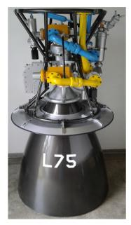
Figure 1. Mockup of L75 engine.
