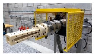
Figure 13. Supersonic combustor coupled to the SCTB using the transition part T-100.
