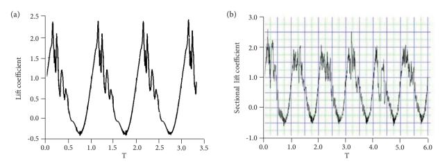
**Figure 5.** Time independency diagram of instantaneous lift coefficient based on dimensionless time in each cycle of oscillation (a) Present research and (b) Wang *et al.* (2010).
