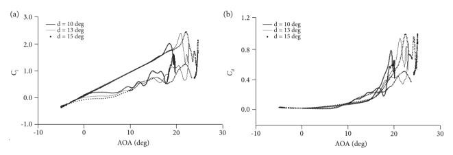
**Figure 12.** Instantaneous aerodynamic coefficients based on the angle of attack for various oscillation amplitudes. (a) Instantaneous lift coefficients; (b) Instantaneous drag coefficient.
