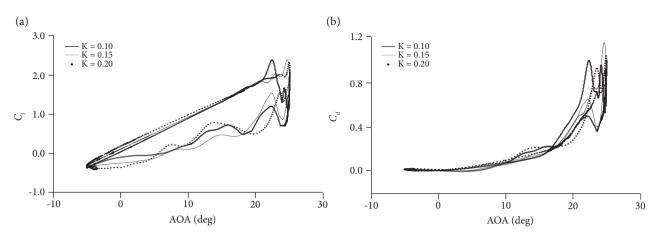
Figure 10. Instantaneous aerodynamic coefficients based on the angle of attack for various reduced frequencies (a) Instantaneous lift coefficients; (b) instantaneous drag coefficients.
