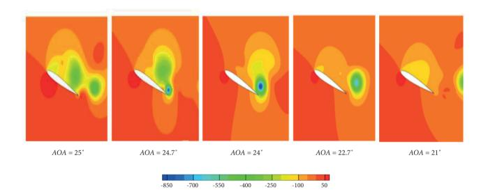
Figure 8. Pressure contour for various angles of attack.
