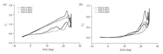
Figure 11. Instantaneous aerodynamic coefficients based on the angle of attack for various airfoil thicknesses. (a) Instantaneous lift coefficients; (b) Instantaneous drag coefficients.
