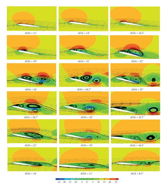
Figure 7. Velocity contour for various angles of attack in a pitching motion condition.
