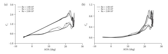
Figure 9. Instantaneous aerodynamic coefficients based on the angle of attack for various Reynolds number. (a) Instantaneous lift coefficients; (b) Instantaneous drag coefficients.
