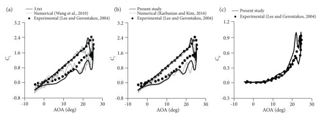
**Figure 6.** Comparison between results of the present simulation with numerical results of Karbasian and Kim (2016), Wang *et al.* (2010) and experimental data of Lee and Gerontakos (2004) (a) and (b) Lift coefficient hysteresis loop; and (c) Drag coefficient hysteresis loop.
