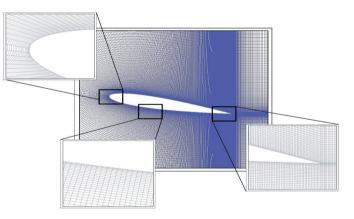
Figure 2. C- type mesh around NACAOO12 airfoil.
