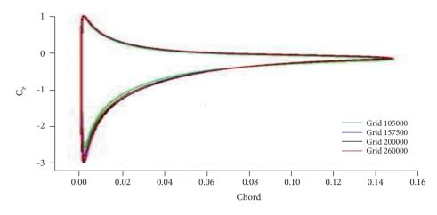
Figure 4. Comparison of pressure coefficient for different cell numbers.
